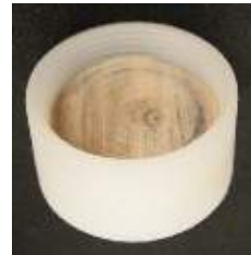
Two-part holder with the xylem filter
