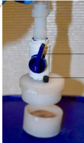
Two-part holder with the xylem filter
